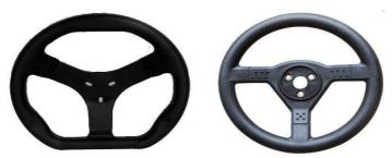
There should not be any external covering to the steering wheel during T.I. If the teams are manufacturing their own metal steering wheel then the minimum pipe outer diameter should be 3/4<sup>th</sup> inch, irrespective of the material type.
